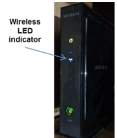
Figure 4 –N300 Router– Front with Power On
