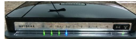
Figure 5 –N750 Router– Front with Power On
